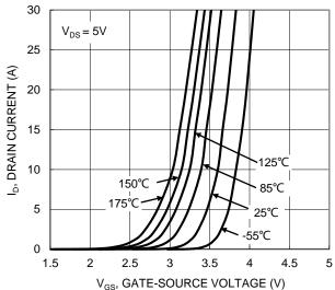
Figure 2. Typical Transfer Characteristic
