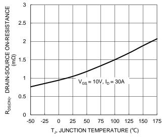
Figure 7. On-Resistance Variation with Temperature
