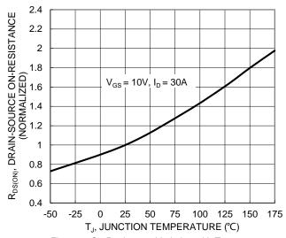
Figure 6. On-Resistance Variation with Temperature
