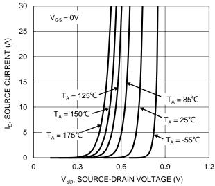
Figure 9. Diode Forward Voltage vs. Current
