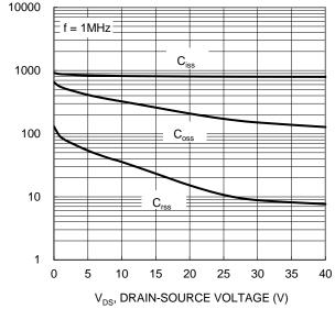
Figure 10. Typical Junction Capacitance
