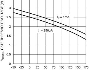
$T_{\rm J},$  JUNCTION TEMPERATURE (°C) Figure 8. Gate Threshold Variation vs. Temperature
