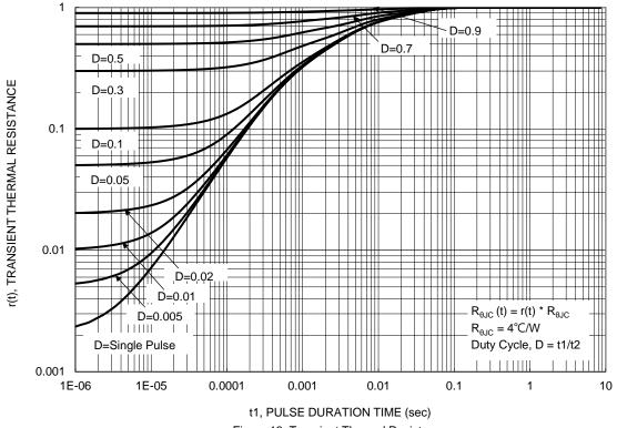
Figure 13. Transient Thermal Resistance
