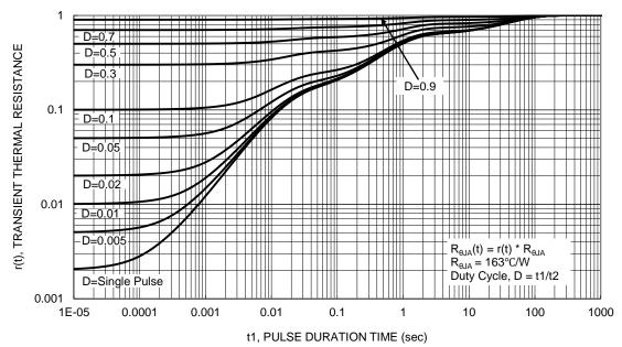
Figure 13. Transient Thermal Resistance
