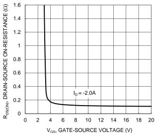
Figure 4. Typical Transfer Characteristic
