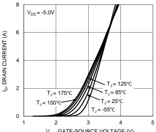
$V_{\text{GS}}$ , GATE-SOURCE VOLTAGE (V) Figure 2. Typical Transfer Characteristic
