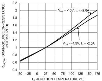
Figure 6. On-Resistance Variation with Temperature
