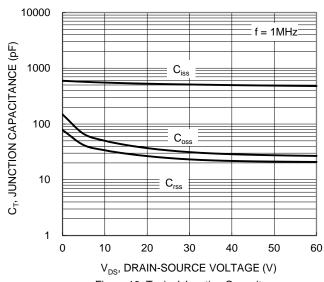
Figure 10. Typical Junction Capacitance
