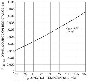
Figure 7 On-Resistance Variation with Temperature
