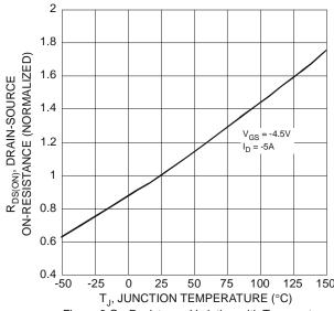
Figure 6 On-Resistance Variation with Temperature
