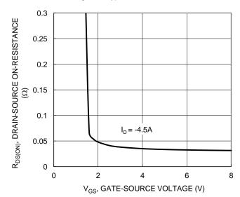
Figure 4. Typical Transfer Characteristic
