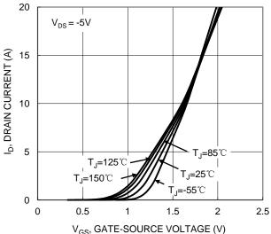
Figure 2. Typical Transfer Characteristic
