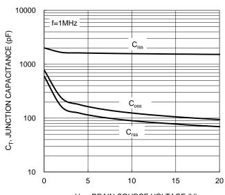
V<sub>DS</sub>, DRAIN-SOURCE VOLTAGE (V) Figure 10. Typical Junction Capacitance
