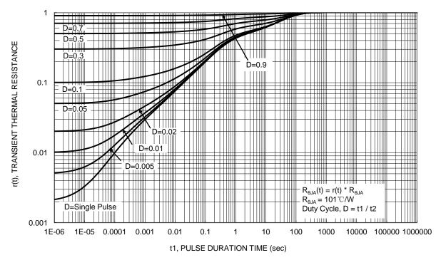
Figure 13. Transient Thermal Resistance
