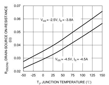
Figure 7. On-Resistance Variation with Junction Temperature
