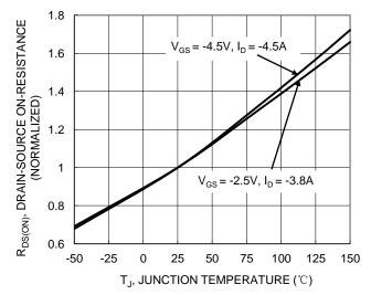
Figure 6. On-Resistance Variation with Junction Temperature
