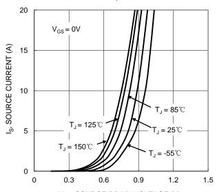
V<sub>SD</sub>, SOURCE-DRAIN VOLTAGE (V) Figure 9. Diode Forward Voltage vs. Current
