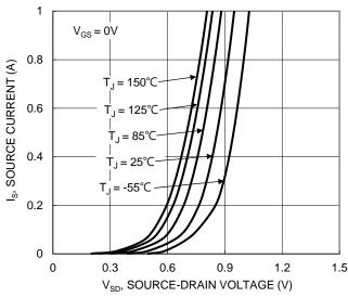
Figure 9. Diode Forward Voltage vs. Current
