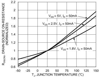
Figure 6. On-Resistance Variation with Junction Temperature
