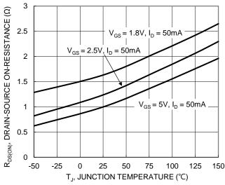
Figure 7. On-Resistance Variation with Junction Temperature
