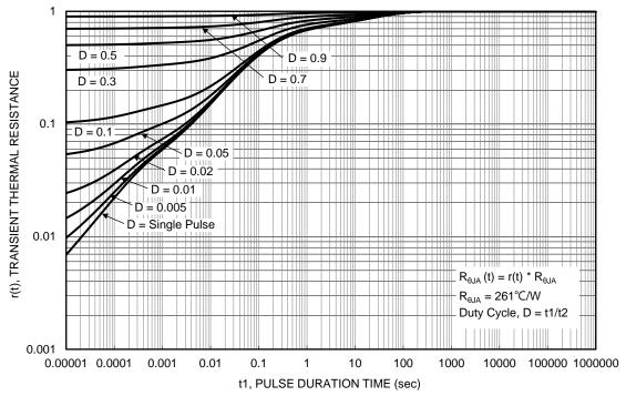
Figure 13. Transient Thermal Resistance
