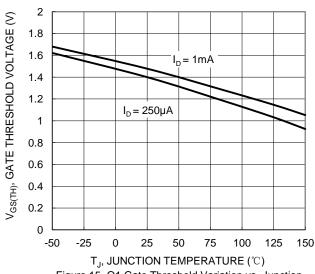
Figure 15. Q1 Gate Threshold Variation vs. Junction Temperature
