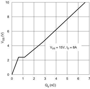
Figure 21. Q1 Gate Charge
