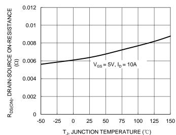
Figure 14. Q2 On-Resistance Variation with Temperature
