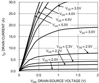
Figure 1. Q1 Typical Output Characteristic
