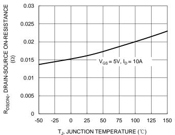
Figure 13. Q1 On-Resistance Variation with Temperature
