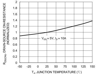
Figure 11. Q1 On-Resistance Variation with Temperature
