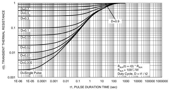
Figure 26. Transient Thermal Resistance
