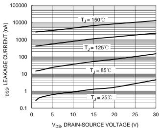
Figure 20. Q2 Typical Drain-Source Leakage Current vs.
