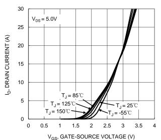
Figure 3. Q1 Typical Transfer Characteristic
