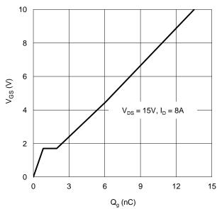
Figure 22. Q2 Gate Charge
