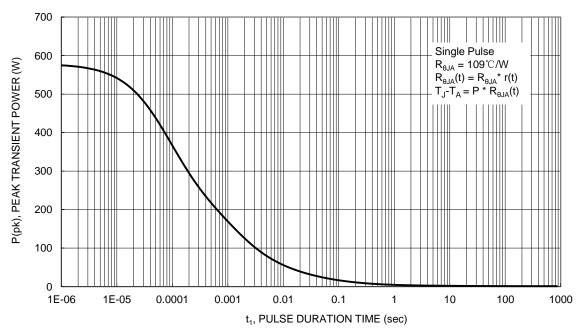
Figure 25. Single Pulse Maximum Power Dissipation
