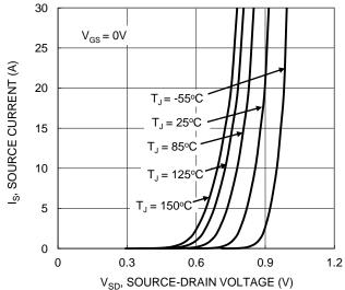
Figure 17. Q1 Diode Forward Voltage vs. Current
