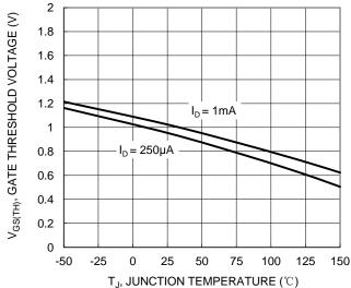
Figure 16. Q2 Gate Threshold Variation vs. Junction Temperature
