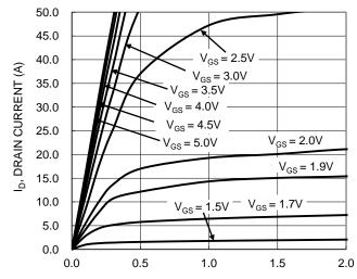
V<sub>DS</sub>, DRAIN-SOURCE VOLTAGE (V) Figure 2. Q2 Typical Output Characteristic
