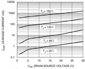
Figure 19. Q1 Typical Drain-Source Leakage Current vs. Voltage
