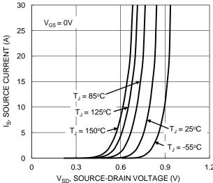
Figure 18. Q2 Diode Forward Voltage vs. Current
