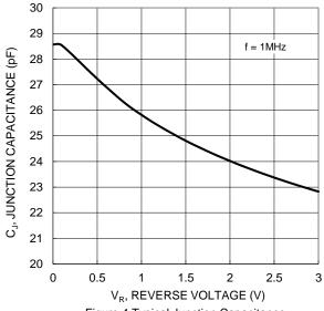
Figure 4 Typical Junction Capacitance
