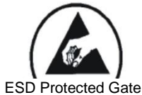
ESD Protected Gate
