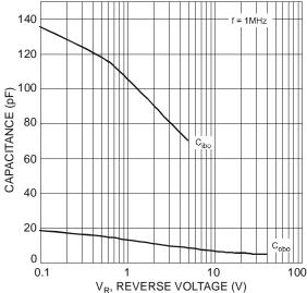
Fig. 6 Typical Capacitance Characteristics
