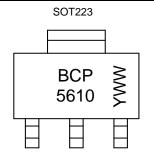
BCP 5610 = Product Type Marking Code YWW = Date Code Marking Y or  $\overline{Y}$  = Last Digit of Year (ex: 9 = 2019) WW or  $\overline{W}W$  = Week Code (01 to 53)
