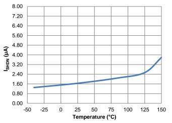
Figure 13. I<sub>SHDN</sub> vs. Temperature
