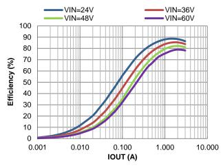
Figure 7. PFM Efficiency vs. Output Current, Vou $\tau$ =3.3V, L=5.5 $\mu$ H
