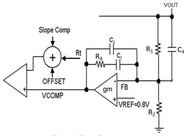
Figure 46. Type 2 Compensator
