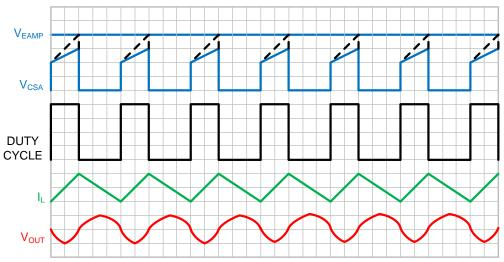
Figure 43. CCM Operation Waveforms
