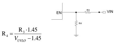
Figure 40. Setting the Input UVLO
