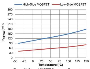
Figure 16. Power MOSFET R<sub>DS(ON)</sub> vs. Temperature
