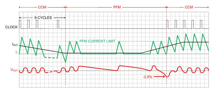
Figure 44. PFM Operation Waveforms
