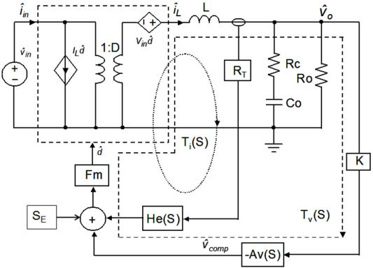
Figure 45. Linearized Small Signal Model
