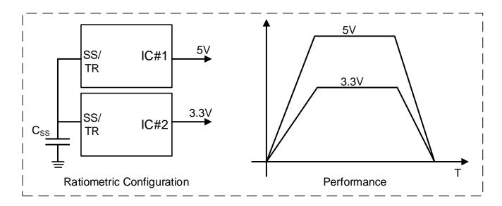
Figure 37. Ratiometic Configuration
