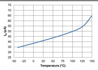
Figure 12. IQ vs. Temperature, IOUT = 0A
