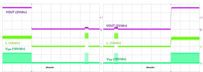
Figure 35. Output Short Protection, IOUT = 3A
