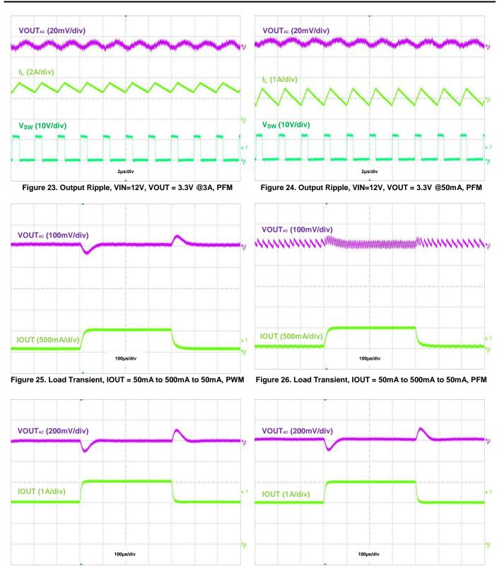
Figure 27. Load Transient, IOUT = 2A to 3A to 2A, PWM
