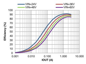
Figure 5. PFM Efficiency vs. Output Current, Vout=5V, L=6.5µH
