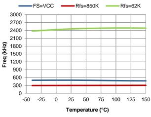
Figure 11. Frequency vs. Temperature
