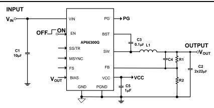
**Figure 1. Typical Application Circuit**
