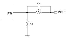
Figure 42. Feedback Divider Network
