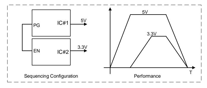
Figure 39. Sequencing Configuration
