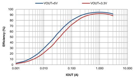
Figure 3. PWM Efficiency vs. Output Current, VIN = 12V,  $f_{sw}$  = 500kHz
