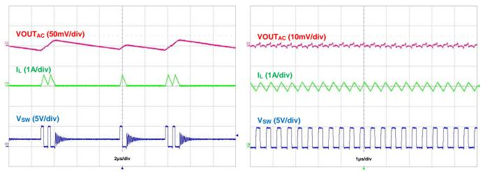
Figure 16. Output Voltage Ripple, IOUT = 50mA
