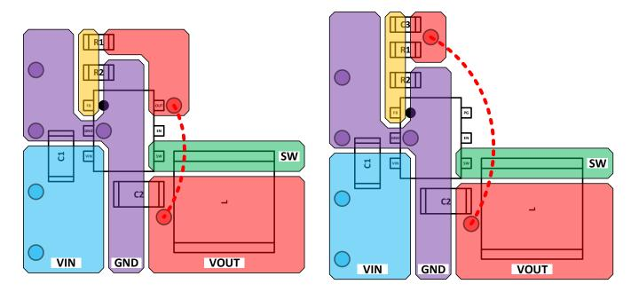
Figure 42. Recommended AP61300Q PCB Layout
