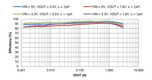
Figure 3. PFM Efficiency vs. Output Current
