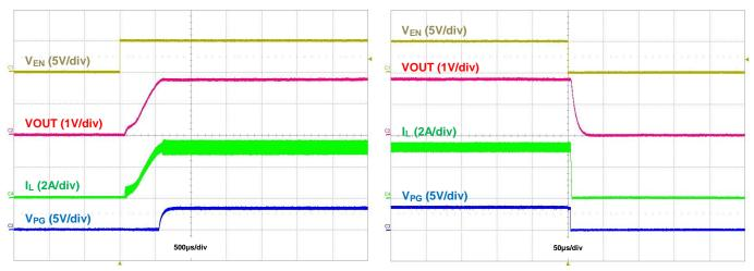
Figure 37. Startup Using EN, IOUT = 3A
