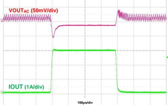
Figure 20. Load Transient, IOUT = 50mA to 3A to 50mA
