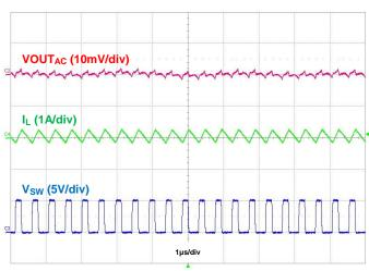
Figure 28. Output Voltage Ripple, IOUT = 50mA
