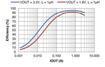
Figure 21. Efficiency vs. Output Current, VIN = 3.3V
