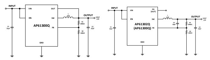
Figure 1. Typical AP61300Q Application Circuit
