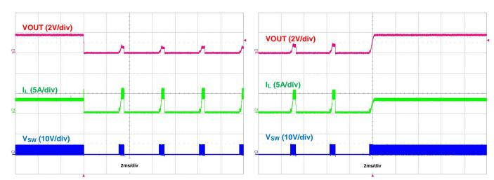
Figure 35. Output Short Protection, IOUT = 3A
