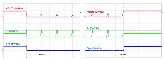
Figure 39. Output Short Protection, IOUT = 3A
