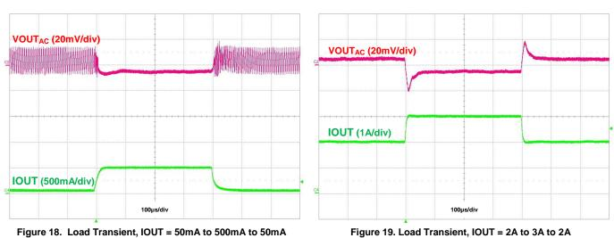
Figure 18. Load Transient, IOUT = 50mA to 500mA to 50mA
