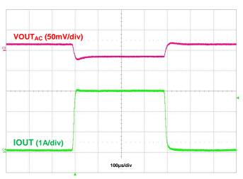
Figure 32. Load Transient, IOUT = 50mA to 3A to 50mA
