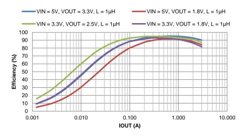
Figure 4. PWM Efficiency vs. Output Current
