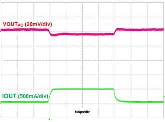
Figure 30. Load Transient, IOUT = 50mA to 500mA to 50mA
