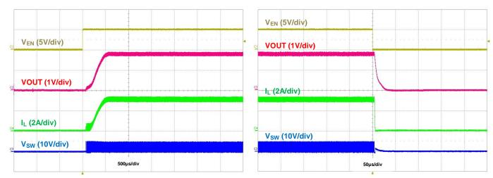
Figure 33. Startup Using EN, IOUT = 3A
