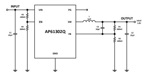
Figure 41. Example Application Circuit for Forced PWM Operation
