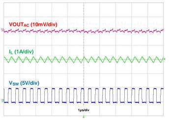
Figure 29. Output Voltage Ripple, IOUT = 3A
