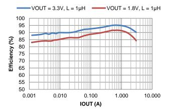
Figure 10. Efficiency vs. Output Current, VIN = 3.3V
