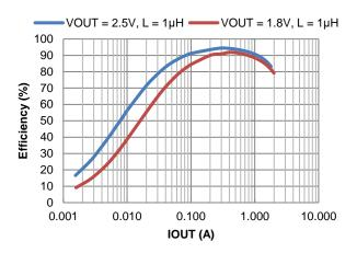
Figure 21. Efficiency vs. Output Current, VIN = 3.3V
