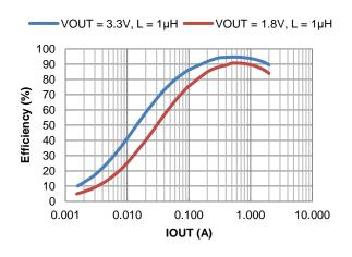
Figure 22. Efficiency vs. Output Current, VIN = 5V
