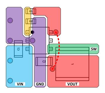
Figure 42. Recommended AP61200/AP61201 PCB Layout
