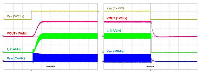
Figure 33. Startup Using EN, IOUT = 2A
