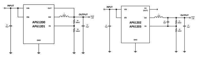
Figure 1. Typical AP61200/AP61201 Application Circuit
