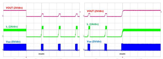
Figure 35. Output Short Protection, IOUT = 2A
