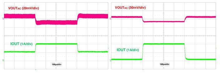
Figure 31. Load Transient, IOUT = 1A to 2A to 1A
