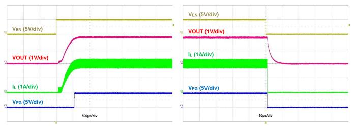
Figure 37. Startup Using EN, IOUT = 2A
