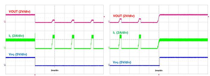
Figure 39. Output Short Protection, IOUT = 2A
