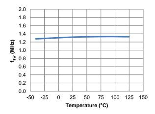
Figure 26. f<sub>SW</sub> vs. Temperature, IOUT = 0A
