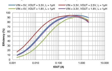
Figure 4. PWM Efficiency vs. Output Current
