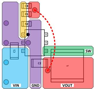
Figure 43. Recommended AP61202/AP61203 PCB Layout
