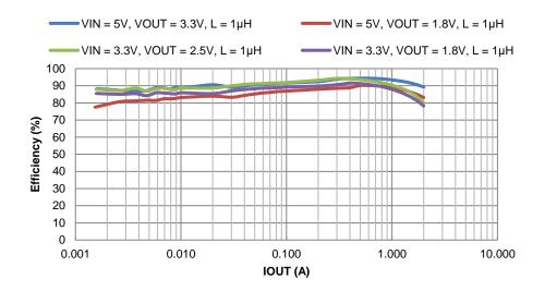
Figure 3. AP61200/AP61202 Efficiency vs. Output Current
