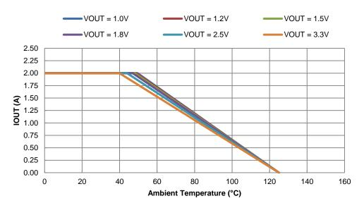
Figure 41. Output Current Derating Curve vs. Ambient Temperature, VIN = 5V
