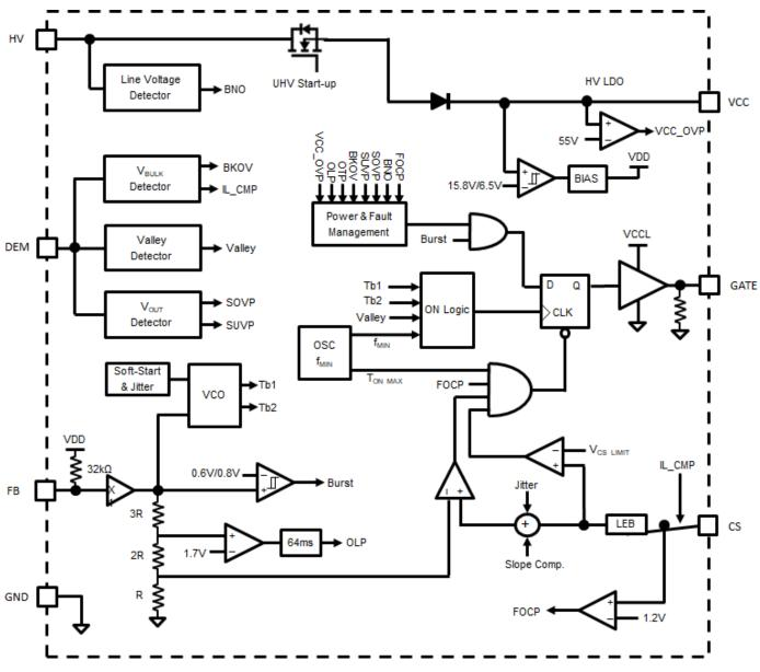
Figure 2. Functional Block Diagram
