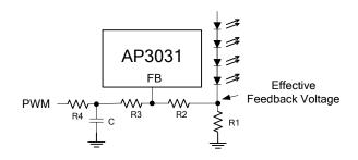
Dimming Control Using Filtered PWM Voltage
