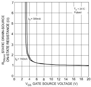
Fig. 6 Static Drain-Source On-Resistance vs. Gate-Source Voltage
