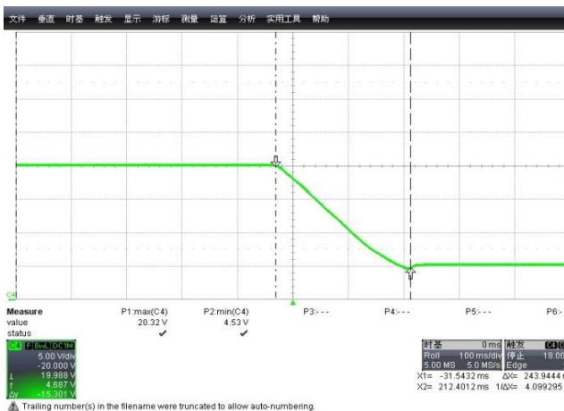
Figure 53: 20V→5.0V Fall Time: 244ms
