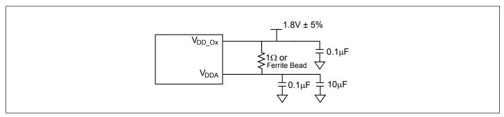
Figure 4. Power Supply Filter
