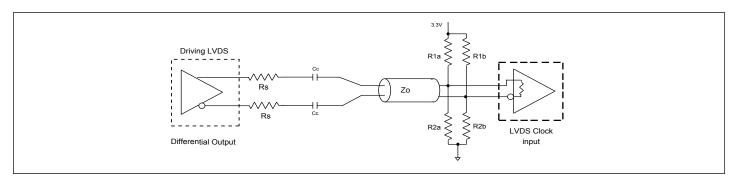
Figure 3. Differential Output driving LVDS
