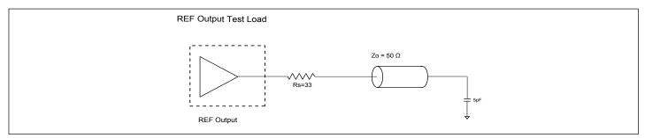
Figure 2. CMOS REF Test Circuit
