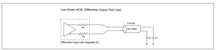
Figure 1. Low Power HCSL Test Circuit
