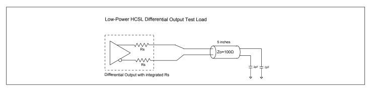
Figure 1. Low Power HCSL Test Circuit
