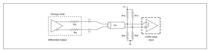
Figure 3. Differential Output Driving LVDS
