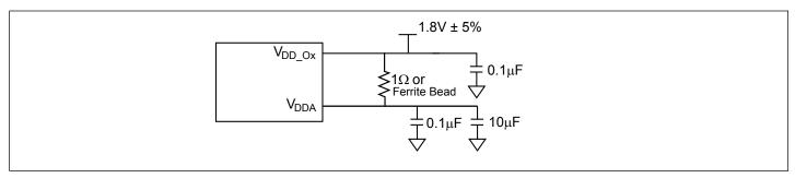
Figure 4. Power Supply Filter
