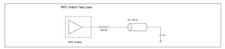
Figure 2. CMOS REF Test Circuit
