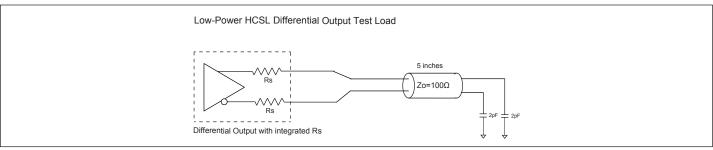
Figure 1. Low Power HCSL Test Circuit
