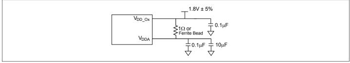
Figure 3. Power Supply Filter
