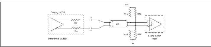
Figure 2. Differential Output Driving LVDS
