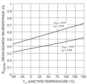
Figure 6 On-Resistance Variation with Temperature
