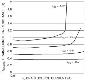
Figure 3 Typical On-Resistance vs.
