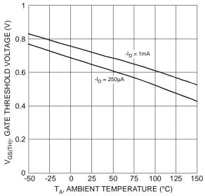
Figure 7 Gate Threshold Variation vs. Ambient Temperature
