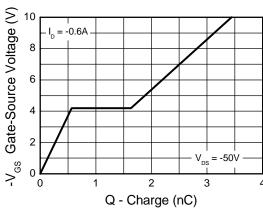
Gate-Source Voltage v Gate Charge
