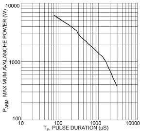
Figure 5 Maximum Avalanche Power Curve, Per Element
