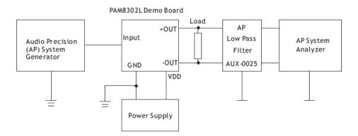
Notes: 1. The Audio Precision (AP) AUX-0025 low pass filter is necessary for every Class-D amplifier measurement with AP analyzer. 2. Two 22µH inductors are used in series with load resistor to emulate the small speaker for efficiency measurement.
