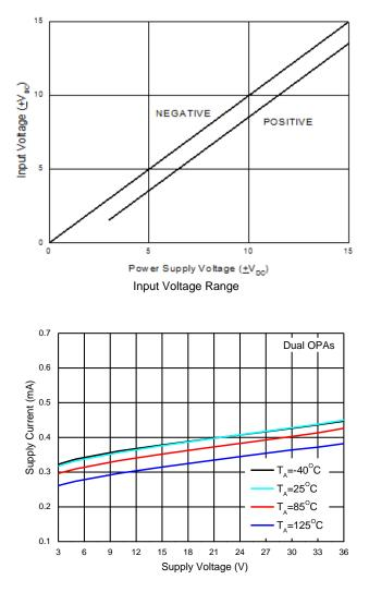
Supply Current vs. Supply Voltage (LM2904Q/LM2904AQ)
