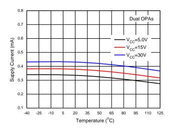
Supply Current vs. Temperature (LM2904Q/LM2904AQ)
