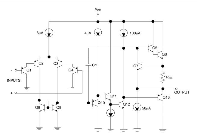
Functional Block Diagram of LM2902Q/LM2902AQ/LM2904Q/LM2904AQ (Each Amplifier)
