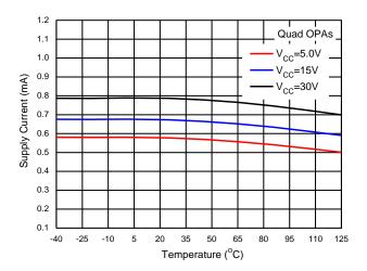
Supply Current vs. Temperature (LM2902Q/LM2902AQ)
