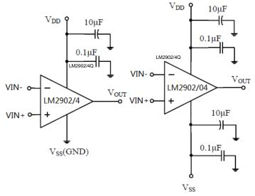
Amplifier with Bypass Capacitors
