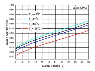
Supply Current vs. Supply Voltage (LM2902Q/LM2902AQ)
