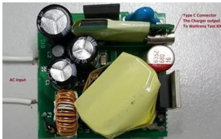
Figure 7: The Sample Board Input & Output Location
