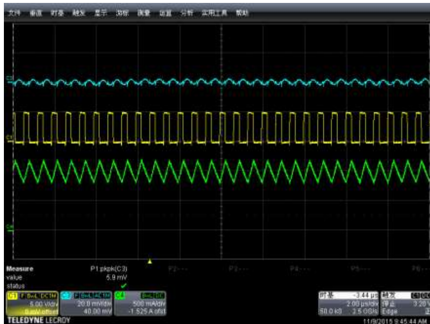
Operation waveform at Iout=1A (Blue-VoutAC; Yellow-Vsw; Green-IL)
