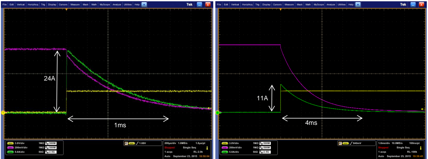
Figure 7 Elevated temperature measurements (approx. T_a=70^{\circ}\text{C} ). Left curves = 24A peak current discharge through DMN3027LFG channel resistance only (200μs/div) Right curves = 11A peak current discharge through DMN3027LFG and 50mΩ series resistor (1ms/div)
