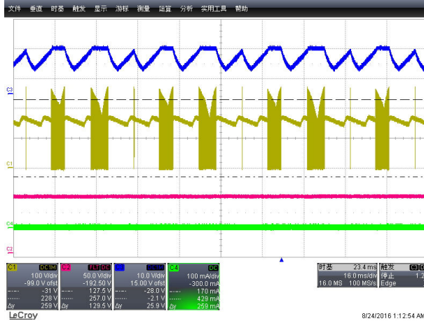
LED Open Protection (Vin=120V AC , Y-V DRAIN , R-V out , B-VCC, G-I LED )
