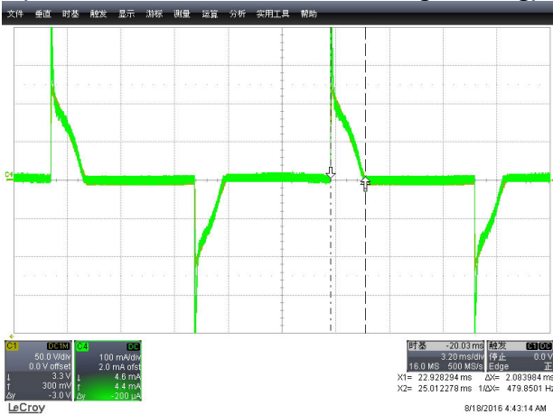
Input AC Current vs Dimmer Phase (Vin=120V AC /60Hz, Conduction angle 45deg)
