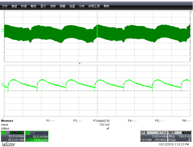
Figure 27: 90Vac/60Hz 20V/2.25A \Delta V=142mV
