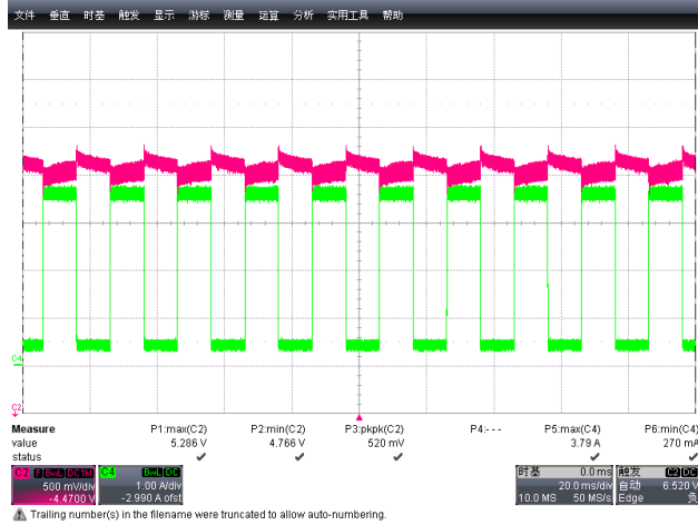
Figure 30: VIN=264VAC, 5V @ 0.4 ~ 3.6A
